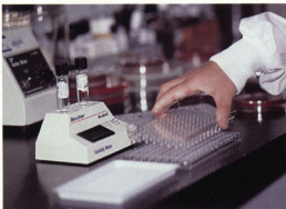
13-12 Broth Microdilution Method—Inoculation of microdilution panel. Microdilution panels are used to quantitatively measure the susceptibility of microorganisms to a battery of antimicrobial agents. The inoculum is mixed and poured into the inoculum/seed tray. The inoculator tips are lowered into the tray and the tips filled by capillary action. The inoculator tips are then lowered into the wells of the panel, as shown here.
