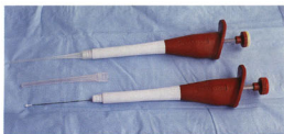
18-10 Positive displacement pipet used in nucleic acid amplification tests (Gilson Medical Electronics, Villiers-le-Bel, France). Amplification methods can result in the production of billions of copies of the same molecule, all concentrated in a very small sample volume. As a result, it is very easy to cross-contaminate specimens during handling of the samples. In order to avoid cross-contamination during pipeting, positive displacement pipets or pipet tips with special filters are used.
