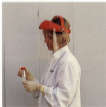
1-10 A full face shield is worn to protect the eyes, nose, and mouth from splashes.
