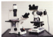
16-1 Microscopes (Olympus Optical Co., Ltd., Japan). A brightfield microscope equipped with epifluorescence is shown on the right and an inverted microscope is on the left. The fluorescence microscope is frequently used in the virology laboratory for the examination of clinical specimens and viruses in culture using immunofluorescent stains. The inverted microscope illuminates the sample from the top with the objectives underneath the specimen. This configuration allows the examination of the cell monolayer from the bottom of the container, while the cells are covered by the nutrient medium. Inverted microscopes are particularly useful for the examination of tissue culture cells in bottles, flasks, miniature plates, and tubes.
