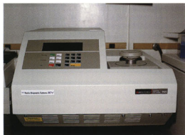
18-13 Automated PCR instrument (Perkin Elmer, Norwalk, Conn.). The system includes a thermocycler and an EIA reader to perform and read the result of a PCR that uses an enzyme-labeled detection system.
