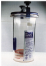
3-23 The GasPak aerobic jar system (Becton Dickinson, Elkridge, Md.) contains a hydrogen and CO 2 generator envelope, a disposable methyl red/blue indicator, and a catalyst holder in the lid.
